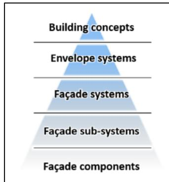
**Figure 2: Vertical decomposition of the façade**
