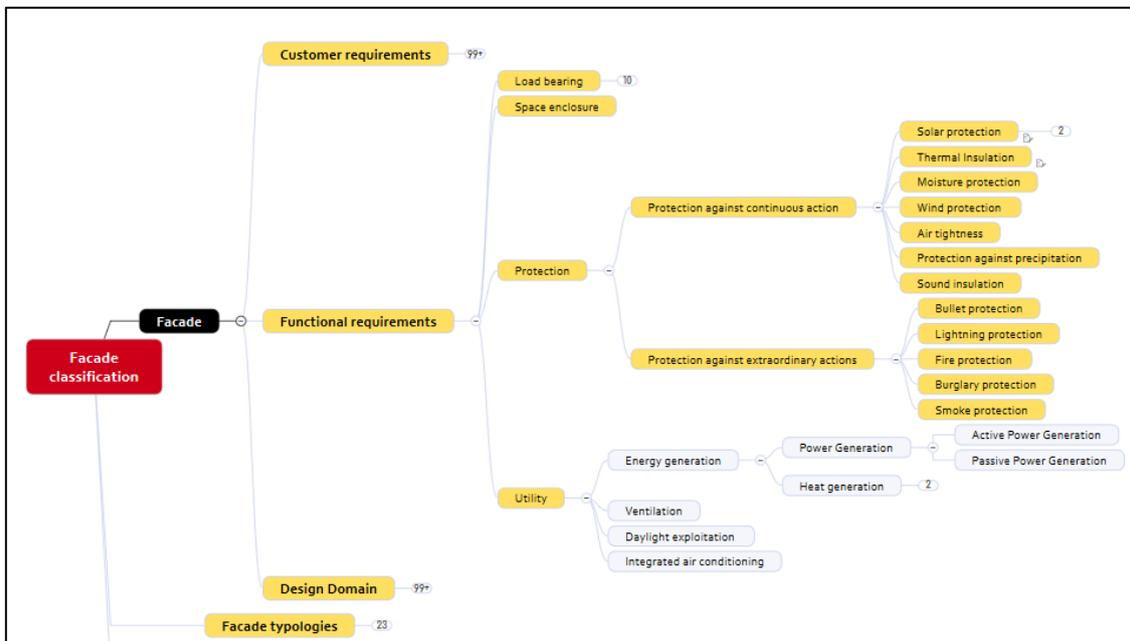
Figure 4c: Extract from the semantic data model of the façade wiki: functional requirements
