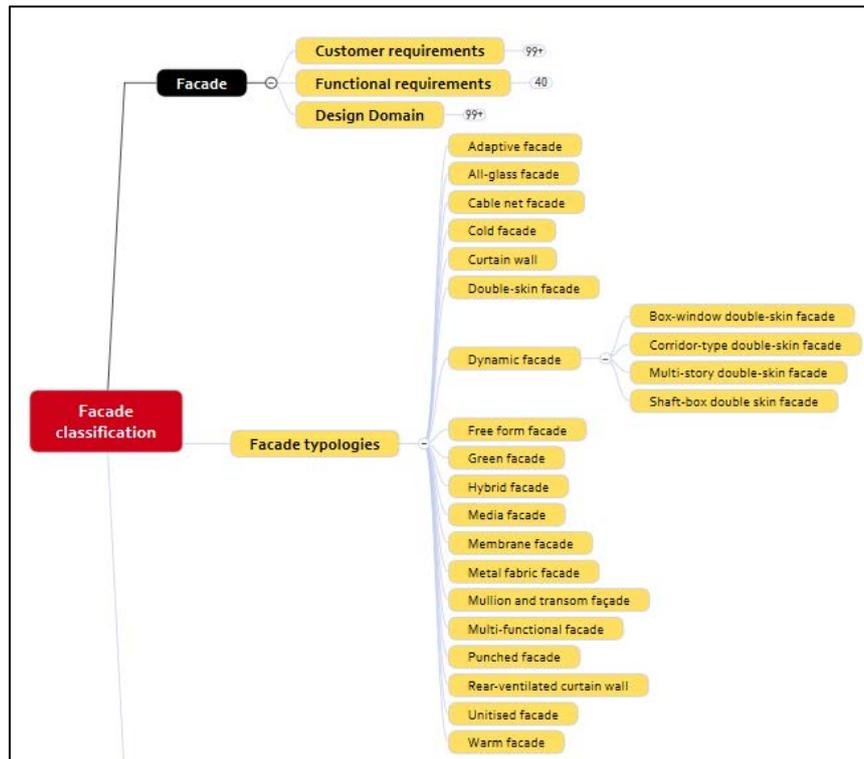
Figure 4d: Extract from the semantic data model of the façade wiki: façade typologies
