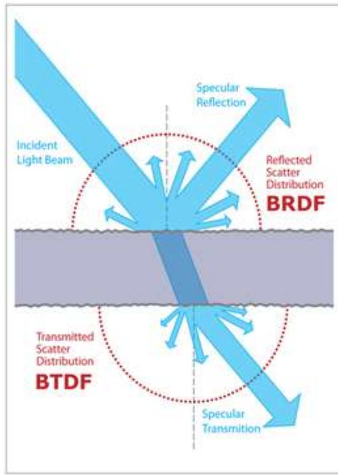
**Figure 2: The composition of a BSDF.  $BSDF = (BTDF + BRDF)$ , BSDF – bidirectional scattering distribution function, BRDF – bidirectional reflection distribution function, BTDF – bidirectional transmission distribution function. (Source: [https://en.wikipedia.org/wiki/Bidirectional\\_scattering\\_distribution\\_function](https://en.wikipedia.org/wiki/Bidirectional_scattering_distribution_function))**
