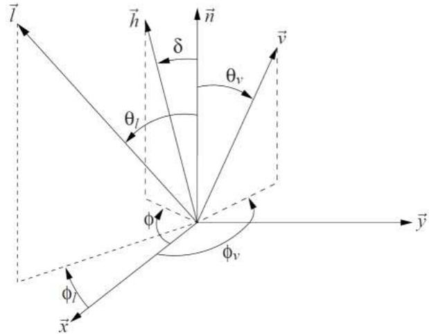
Figure 3: : Diagram showing vectors used to define the BSDF
