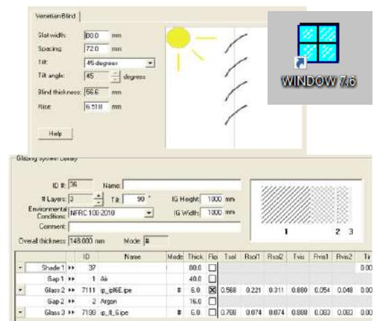
**Fig. 2: Glazing + shading system setup in WINDOW7**
