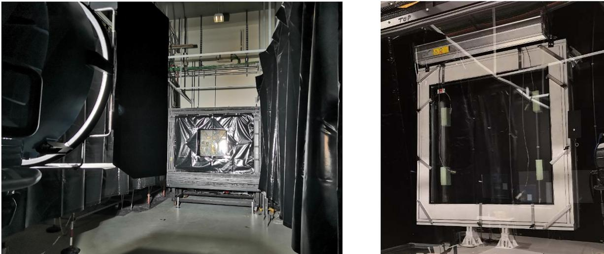
**Figure 10. Left: g-value measuring system at Eurac with activated solar simulator, sample and climatic chamber, right: metering box inside the climatic chamber.**
