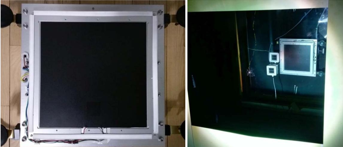
**Figure 8: Prototype with absorbing foil (L) installation in calorimetric test stand at BB (R)**
