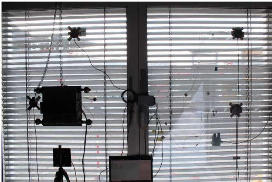
**Figure 4:** Measurement setup from inside showing: thermocouples for the temperature measure of glazing surfaces, blinds and air, a pyranometer measuring the transmitted vertical irradiance, small heat flux sensors shielded from direct solar irradiance, conventional heat flux plates and a temperature-controlled in-situ measurement device to determine the undisturbed, transient heat flux through transparent components.
