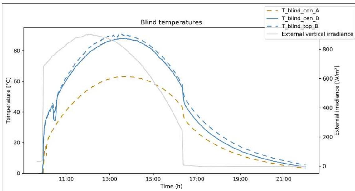
**Figure 6: Blind temperatures for the two façade samples on a clear sky day; sensors named “cen” are positioned on a blind at the centre of the window, sensors named “top” are positioned at a distance of  $\frac{1}{4}$  of the total height from the upper limit; open cavity.**
