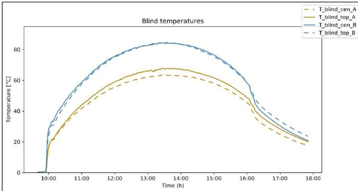
**Figure 5: Blind temperatures for the two façade samples on a clear sky day; sensors named “cen” are positioned on a blind at the centre of the window, sensors named “top” are positioned at a distance of  $\frac{1}{4}$  of the total height from the upper limit; closed cavity**
