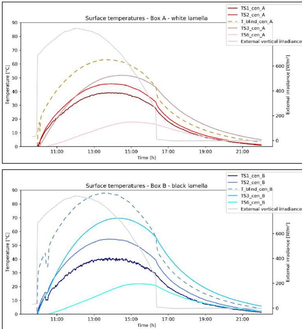
**Figure 8: Surface temperatures of façade sample A (top) and B (bottom). Detail of glazing centre-of-glass surface and blinds temperatures. Open cavity configuration. TS1 = face 1, TS2 = face 2, TS3 = face 3, TS6 = face 6. (Face 4 and 5 are the internal faces in the IGU).**
