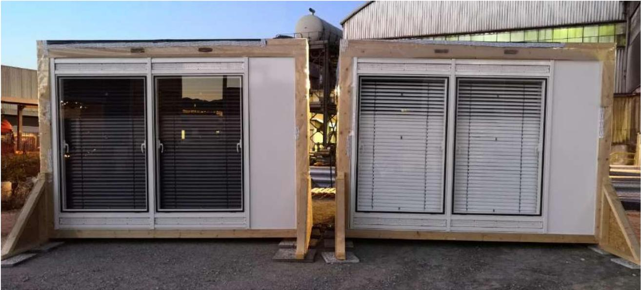
**Figure 2: Front view of the two façade samples, right: sample A with externally white blinds, left: sample B with externally black blinds.**
