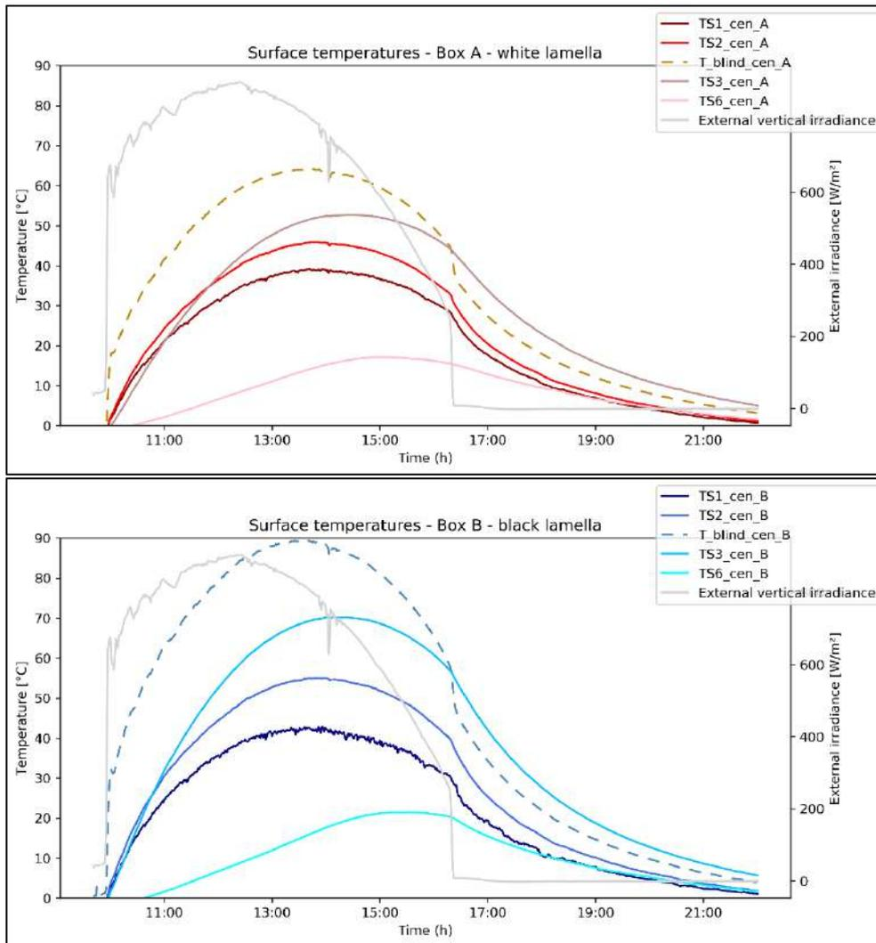
**Figure 7: Surface temperatures of façade sample A (top) and B (bottom). Detail of glazing centre-of-glass surface and blinds temperatures. Closed cavity configuration. TS1 = face 1, TS2 = face 2, TS3 = face 3, TS6 = face 6. (Face 4 and 5 are the internal faces in the IGU).**
