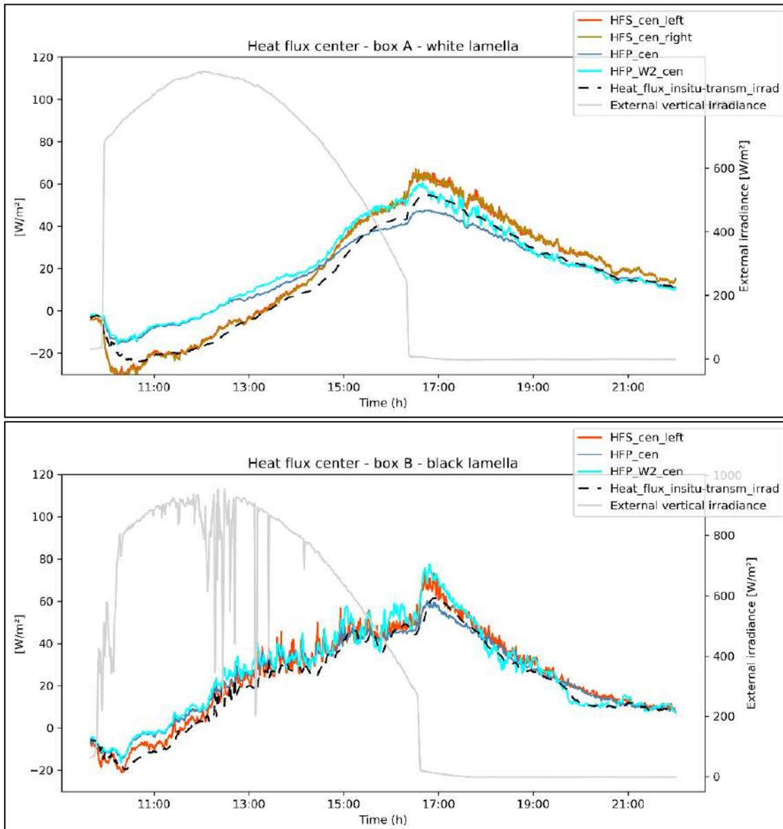
**Figure 12: Heat flux measured at the centre of the room-side glazing surface; heat flux sensors (HFS), heat flux plates (HFP), temperature-controlled in-situ heat flux device minus transmitted irradiance (Heat\_flux\_insitu-transm-irrad) - Open cavity.**
