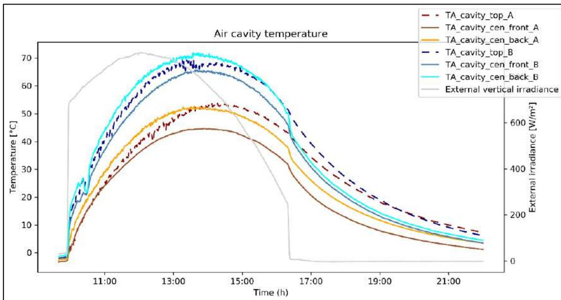
Figure 10: Air cavity temperatures for façade sample A and B – open cavity.
