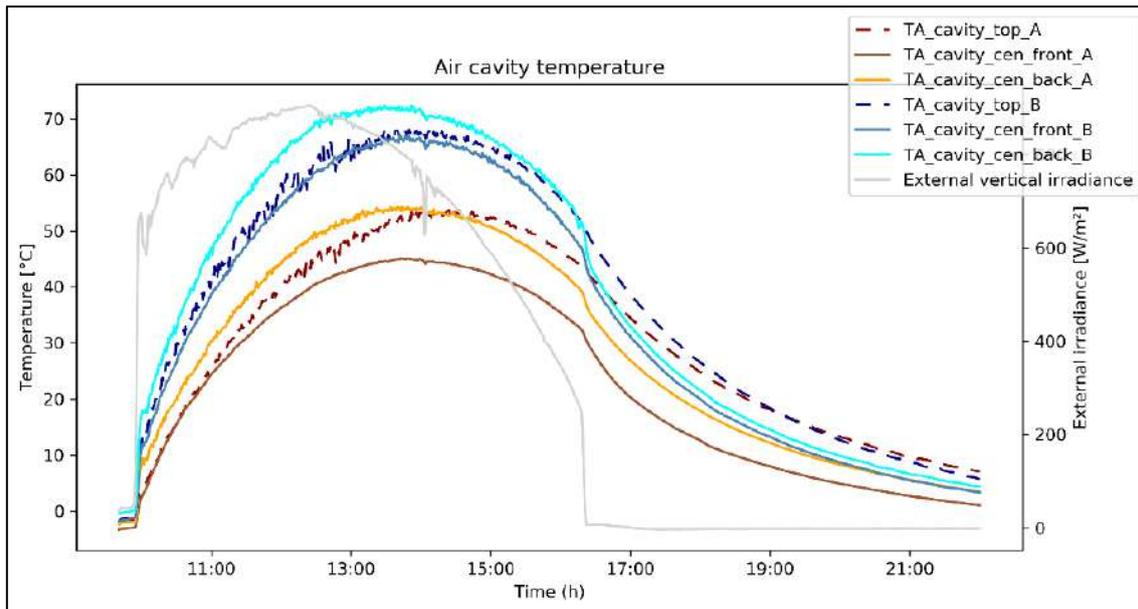
Figure 9: Air cavity temperatures for façade sample A and B – closed cavity
