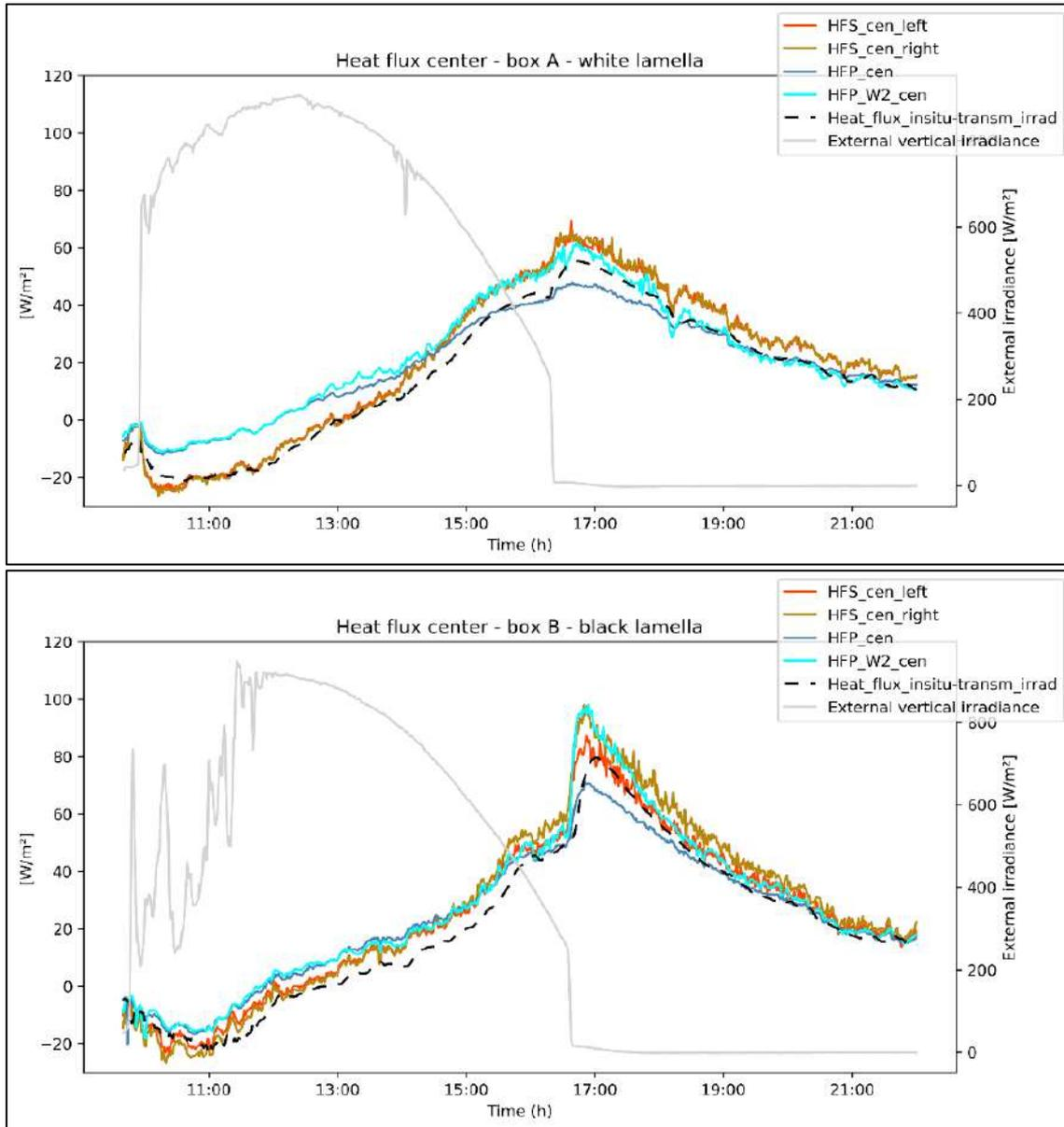
**Figure 11: Heat flux measured at the centre of the room-side glazing surface; heat flux sensors (HFS), heat flux plates (HFP), temperature-controlled in-situ heat flux device minus transmitted irradiance (Heat\_flux\_insitu-transm-irrad) - Closed cavity**
