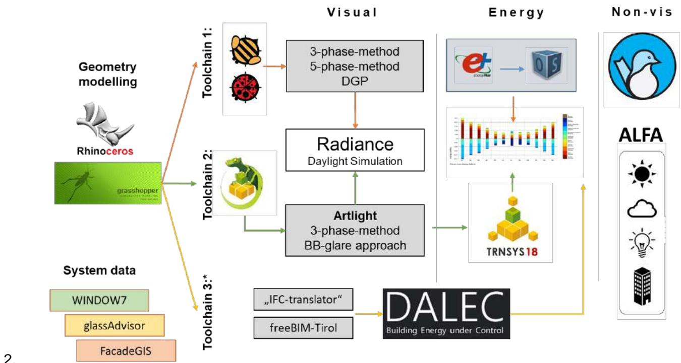
Figure 16: FACEcamp simulation toolchain for complex facade systems
