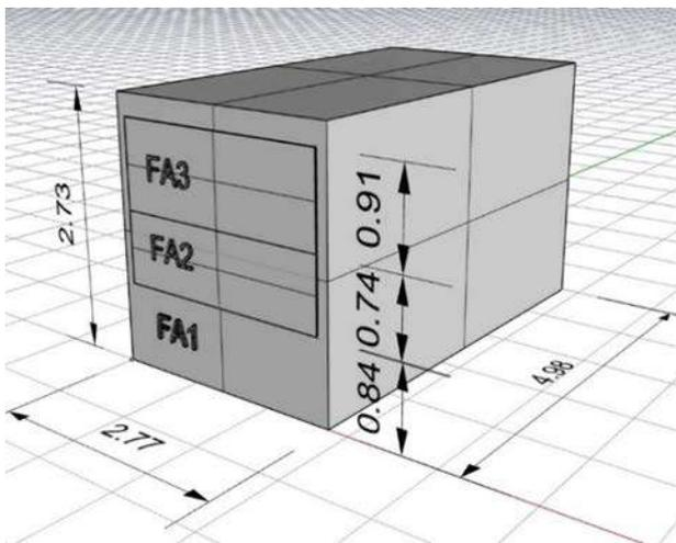
Figure 7: Sketch of the PASSYS test cell model in Rhinoceros
