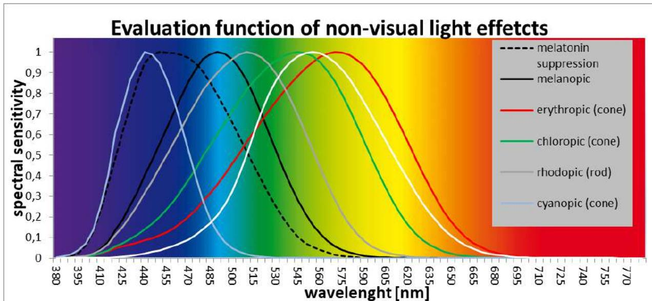
**Figure 2: Absorption spectra of the human cones and rods; additionally the action spectra of acute nighttime melatonin suppression and the photopigment melanopsin and the human light sensitivity curve ( $V(\lambda)$ ) are shown. Source: DIN 5031-100 (2009)**
