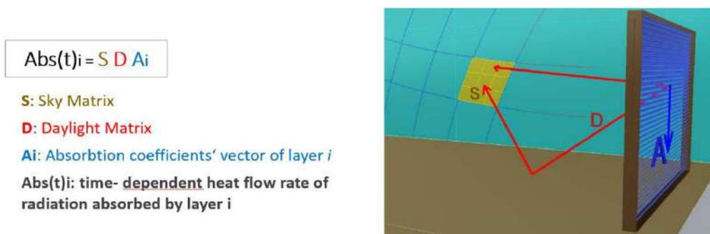
**Figure 7: Schematic representation of the “modified Three-Phase Method”.**
