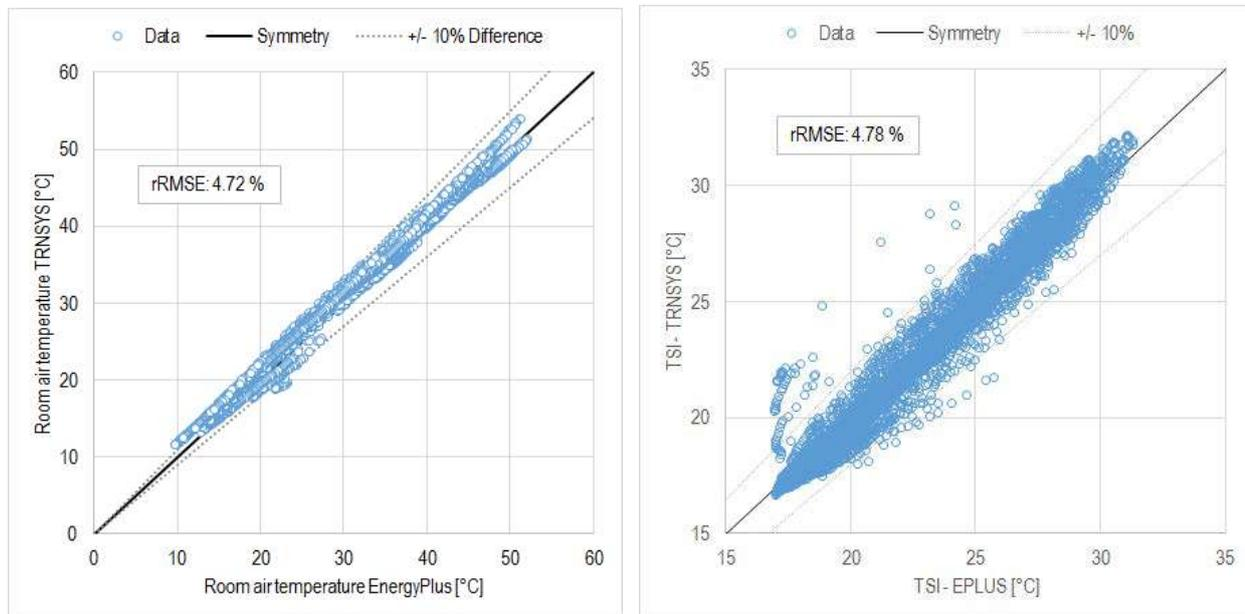
**Figure 4: Comparison of sensitive room air temperature (left) and glazing surface temperature (right)**
