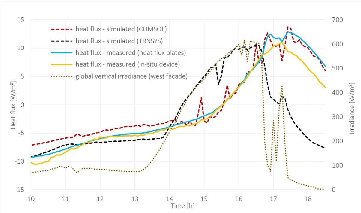
**Figure 9: Comparison of simulated and measured heat flux through the CFS.**
