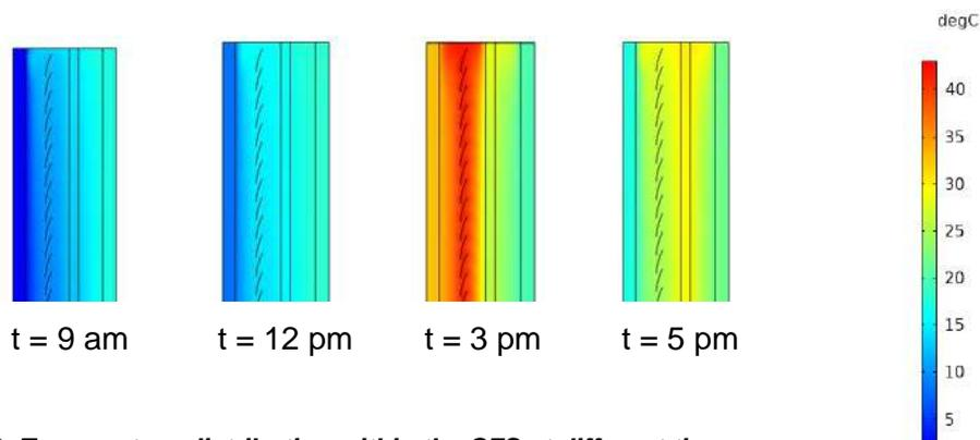
**Figure 10: Temperature distribution within the CFS at different times**
