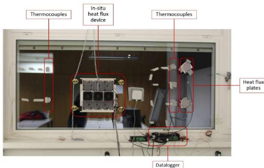
**Figure 8: Measurement setup for the CFS**
