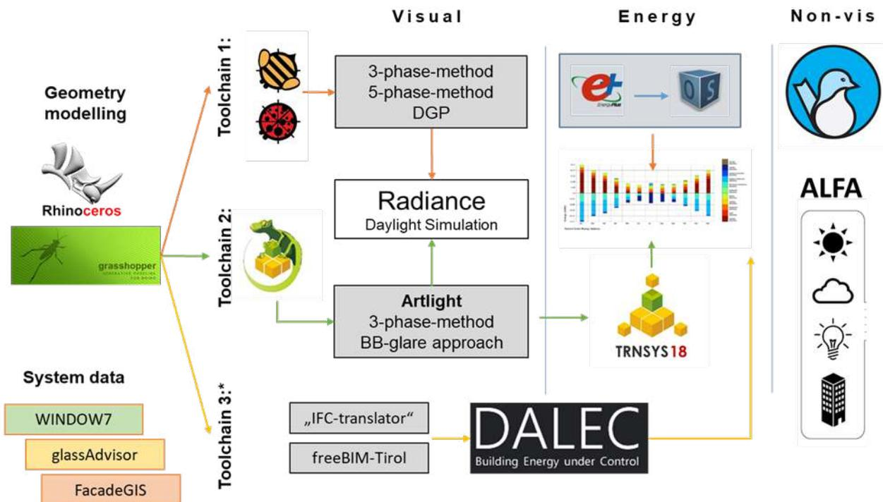
**Figure 1: FACEcamp simulation toolchain for complex facade systems**
