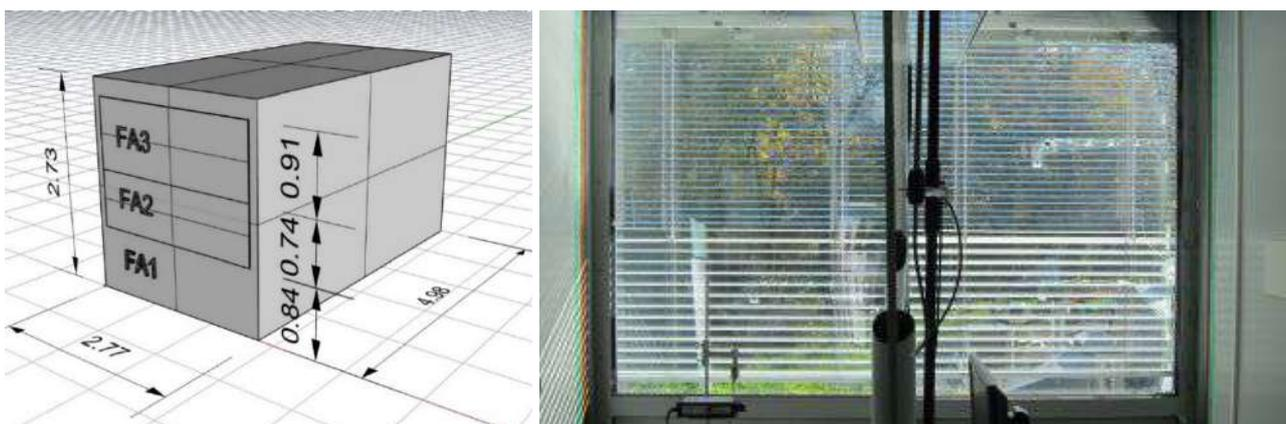
**Figure 3: Sketch of the PASSYS test cell model in Rhinoceros (left); Installed facade at PASSYS-cell (right)**
